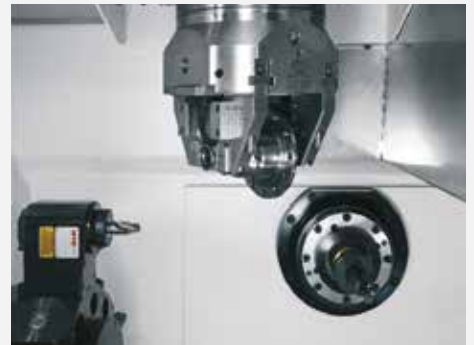
The integrated milling spindle allows internal processing of differential housings in one set-up
