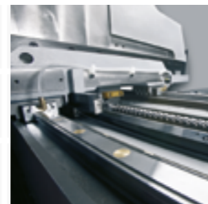
Highest precision: Glass scales and digital drive technology allow high acceleration and contour accuracy.
